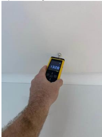
High moisture readings.
